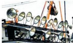
In action: The lights of a purse seiner, which attracts fish towards the nets in the fishing boat.
